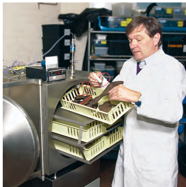
Fig.1564 The freeze-drier in use with leather
